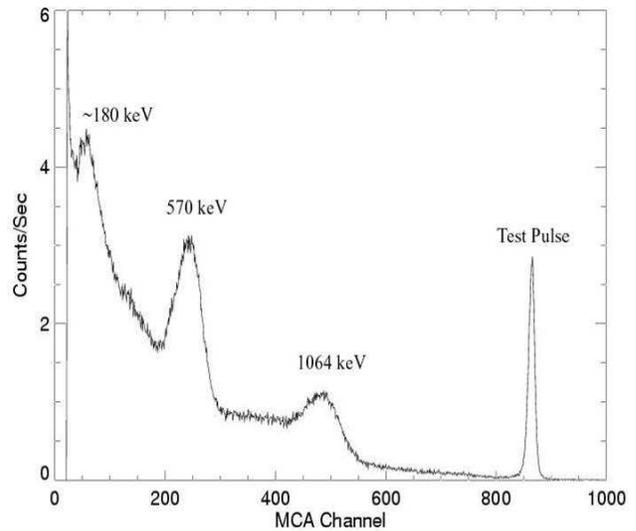
Figure 7. Typical charge spectrum from Bi-207.
