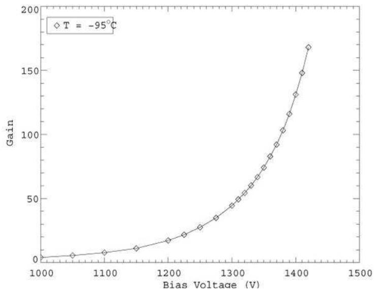
Figure 4. Gain versus bias voltage on LAAPD.
