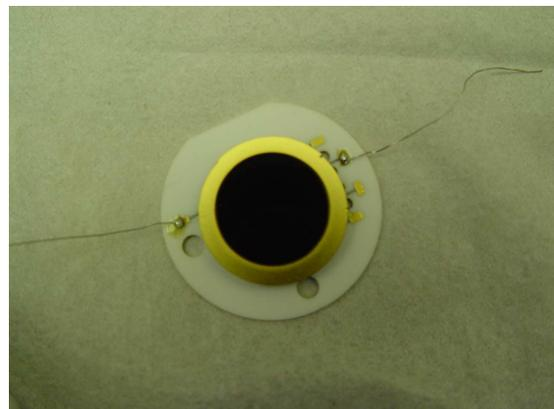
Fig. 1. 16mm diameter LAAPD from Advanced Photonix.
