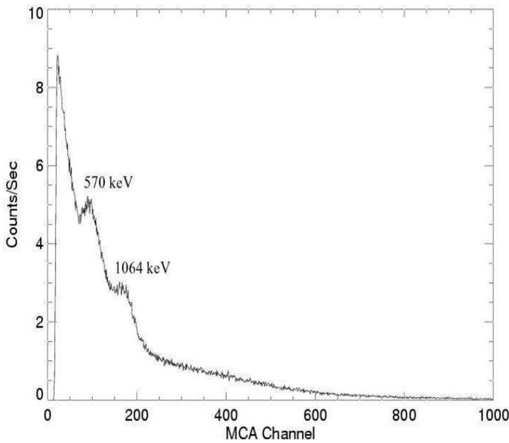
Figure 5. Typical light spectrum from Bi-207.
