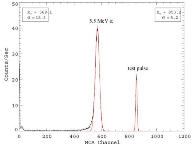
Figure 8. Typical charge spectrum from Am-241.
