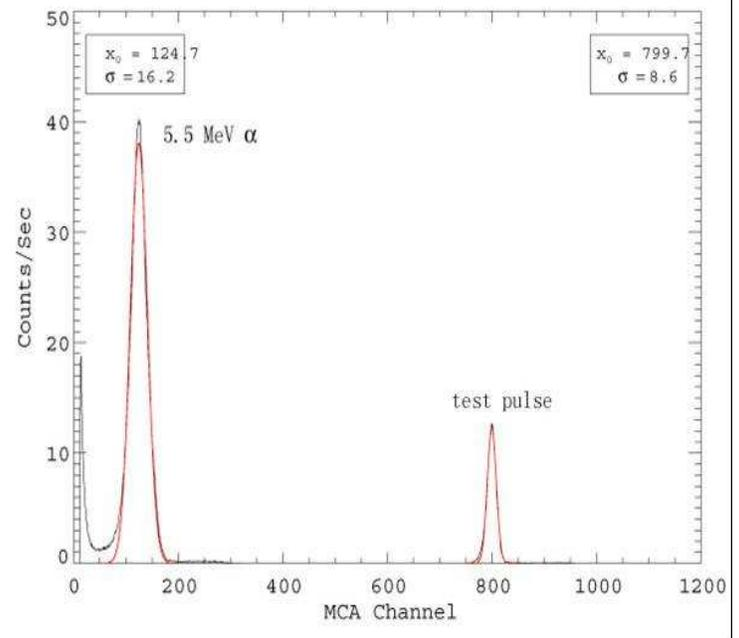
Figure 6. Typical light spectrum from the Am-241 source.
