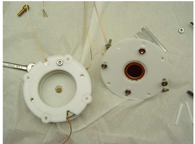
Fig. 2. Right- Teflon housing with LAAPD. Left- Charge Collection and Anode Grid in Teflon housing.
