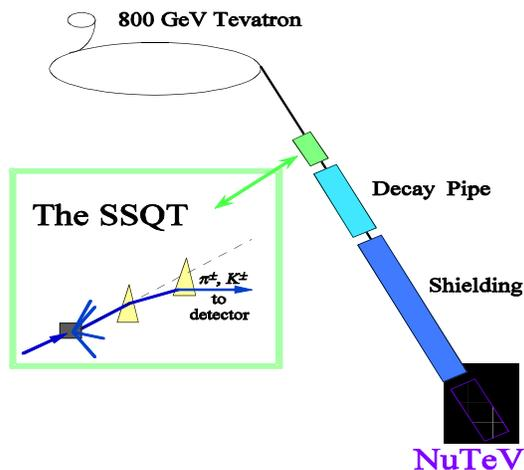
Illustration 4: Schematic of the NuTeV beam
