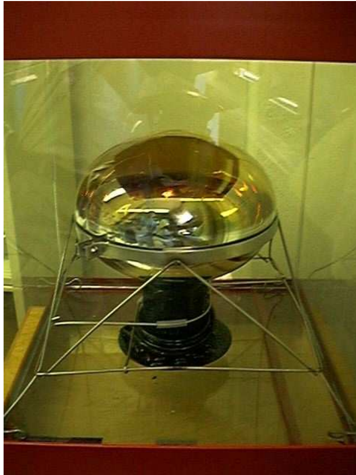
Figure 1: A typical phototube used in the MiniBooNE detector: an 8 inch R1408 mounted on its wire frame. The base is coated with Masterbond before the PMT is installed into the detector.
