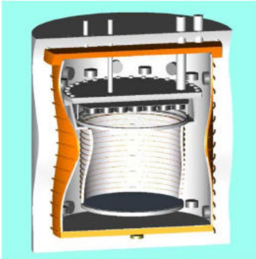
Fig. 7 Schematic view of the XENON 100 dual phase detector
