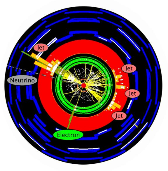
This is the top view of the W boson and 4 jets event. This view is slightly more ambiguous because along the center line there appear to be jets (in addition to the labeled jets). This is because the protons' other constituents not involved in the collision may collide as well, but their collisions are usually considered more glancing and less head-on.
