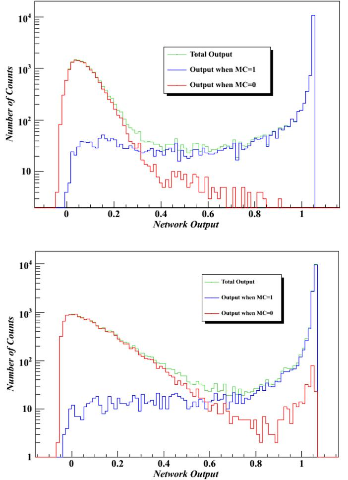
Figure 3. Histograms displaying network response for different expected outputs from the full training set NN (top) and the limited training set NN (bottom).
