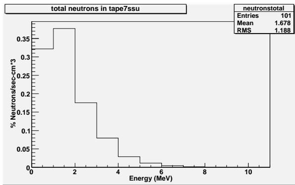
FIG. 8: The spontaneous fission neutron spectrum and the alpha-neutron spectrum combined to create a total neutron spectrum.
