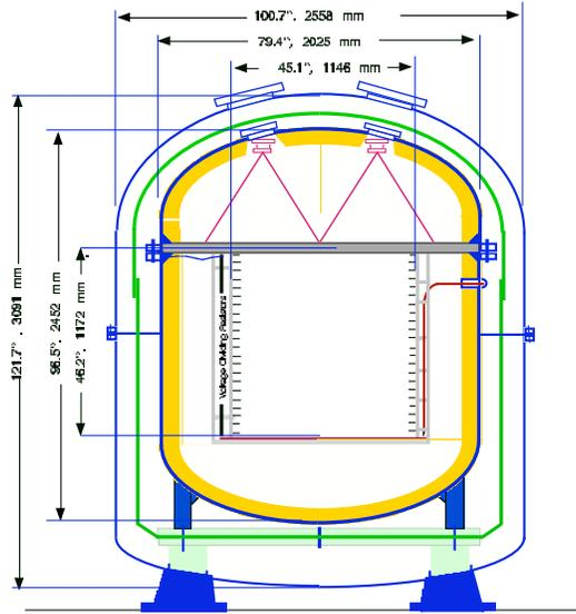
FIG. 2: The schematics of our meter cubed proof of concept prototype.
