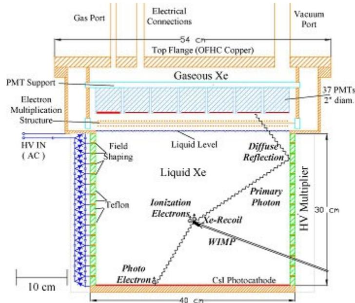
Figure 2.1: Diagram of the XENON100 detector
