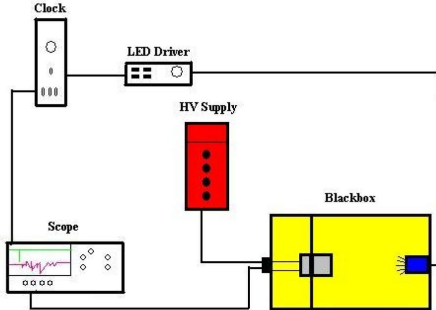
Figure 3.3: PMT calibration setup.
