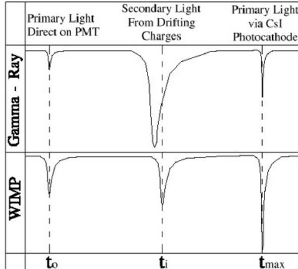
Figure 3.1: Signal differences between an electron recoil event and a nuclear recoil event
