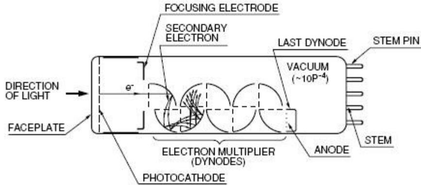
Figure 3.2: PMT construction
