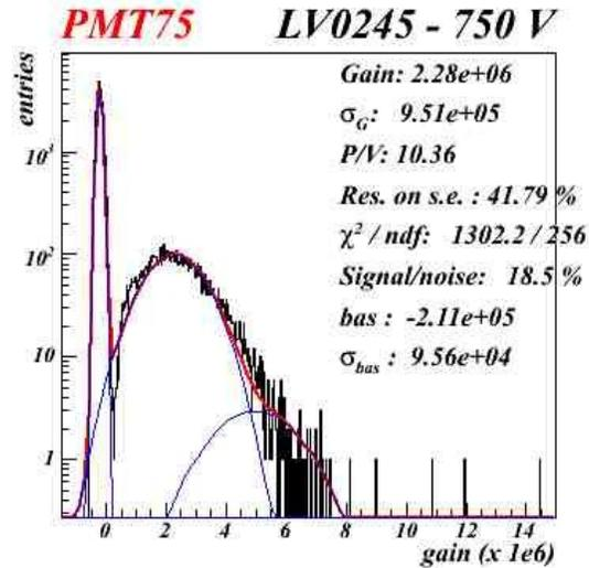
Figure 4.1: PMT calibration data on PMT 75, located in the top array taken on July 27, 2008.
