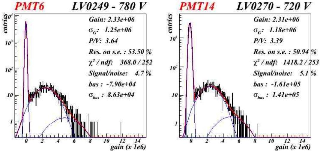
Figure 4.2: Calibration comparison for PMT 6 and PMT 14 on the top array taken on July 27, 2008.
