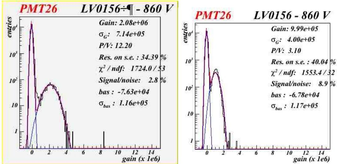
Figure 4.4: Calibration results for PMT 26. The PMT is shown to be functioning at a gain of around  $2e6$  on June 27 (left) and when tested 3 weeks later on July 16 it shows a gain of only  $\sim 1e6$ .
