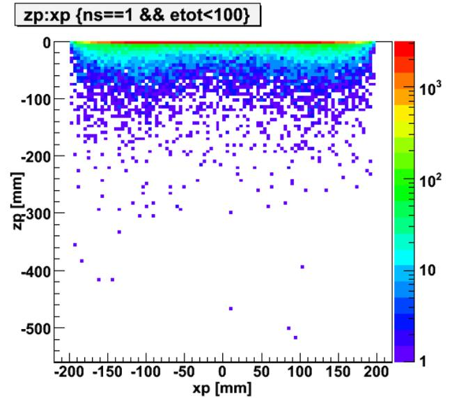
Figure 6. Monte Carlo simulation of events distribution for top PMTs in the current design of XENON100 upgrade of z position vs x position with a target volume cut, single scatter cut, and veto energy less than 100keVee cut.
