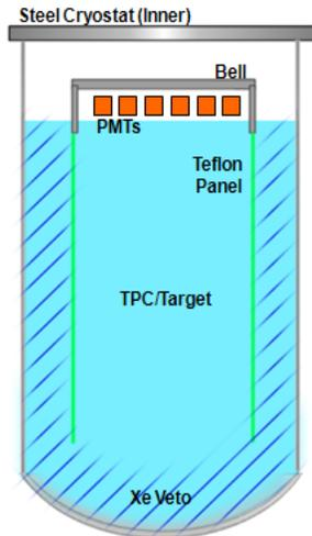
Figure 12. Original detector setup (conceptually) in Monte Carlo simulation, not to scale. Copper outer vessel of the cryostat is not shown, but was included in the simulation.
