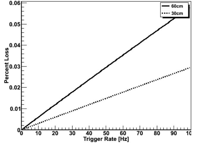
Figure 2. Dead time loss as a function of the true interaction rate for a drift length of 60 cm (Upgrade) and 30 cm (XENON100).
