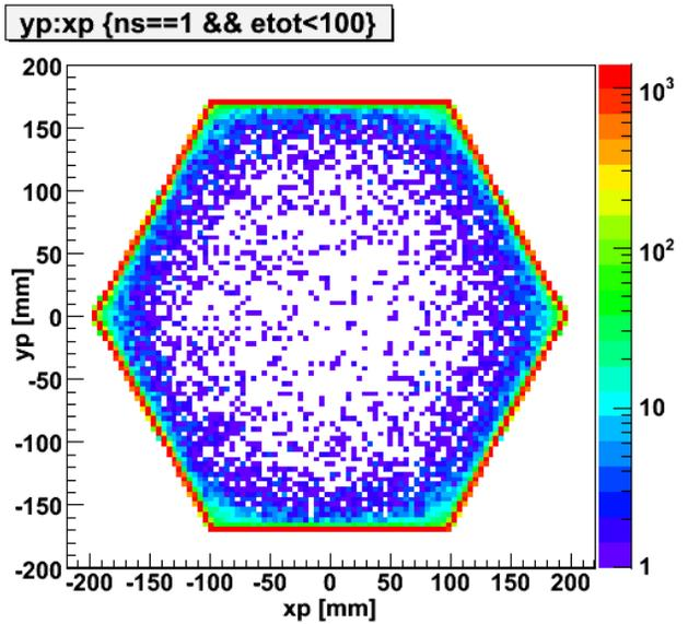
Figure 8. Monte Carlo simulation of events distribution for Teflon in the current design of XENON100 upgrade of y position vs x position with a target volume cut, single scatter cut, and veto energy less than 100keVee cut.
