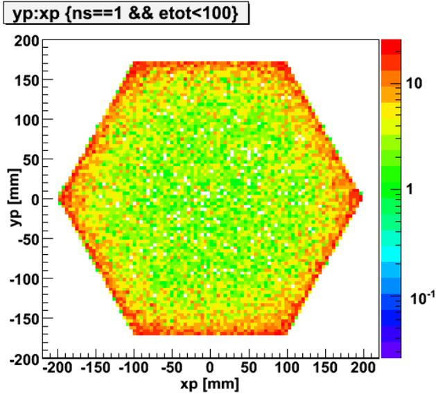
Figure 7. Monte Carlo simulation of events distribution for steel in the current design of XENON100 upgrade of y position vs x position with a target volume cut, single scatter cut, and veto energy less than 100keVee cut.
