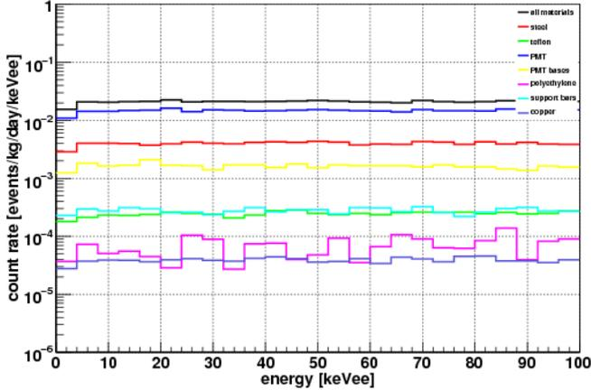
Figure 1. Energy spectrum of simulated gamma background in XENON100 (Alexander Kish), with a 50kg fiducial volume cut.
