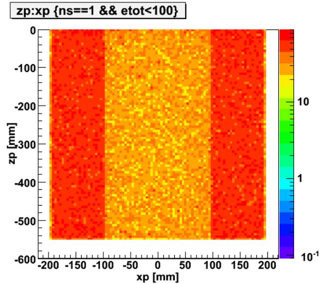
Figure 10. Monte Carlo simulation of events distribution for Teflon in the current design of XENON100 upgrade of z position vs x position with a target volume cut, single scatter cut, and veto energy less than 100keVee cut.
