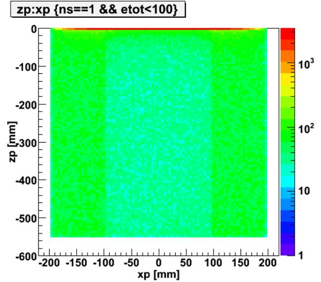
Figure 5. Monte Carlo simulation of events distribution for all materials in the current design of XENON100 upgrade of z position vs x position with a target volume cut, single scatter cut, and veto energy less than 100keVee cut.
