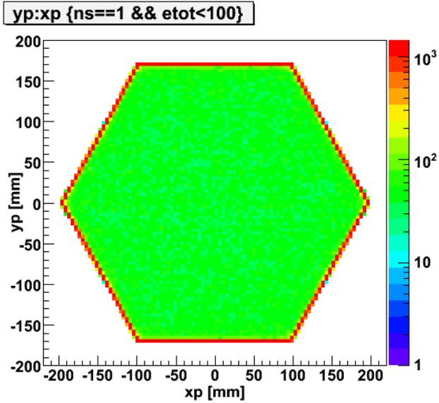
Figure 3. Monte Carlo simulation of events distribution for all materials in the current design of XENON100 upgrade of y position vs x position with a target volume cut, single scatter cut, and veto energy less than 100keVee cut.
