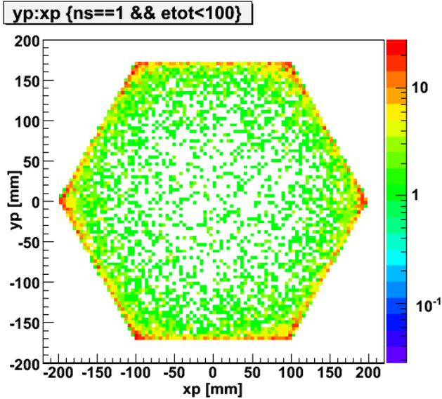
Figure 11. Monte Carlo simulation of events distribution for copper in the current design of XENON100 upgrade of y position vs x position with a target volume cut, single scatter cut, and veto energy less than 100keVee cut.
