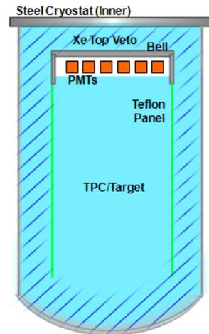
Figure 14. Second detector setup (conceptually) in Monte Carlo simulation, not to scale. Copper outer vessel of the cryostat is not shown, but was included in the simulation. The liquid xenon active veto and xenon gas inside the bell are now included.
