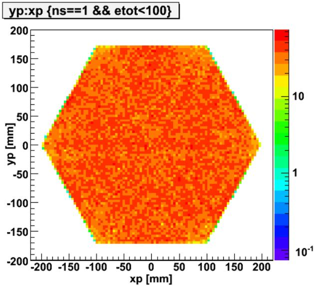
Figure 4. Monte Carlo simulation of events distribution for top PMTs in the current design of XENON100 upgrade of y position vs x position with a target volume cut, single scatter cut, and veto energy less than 100keVee cut.
