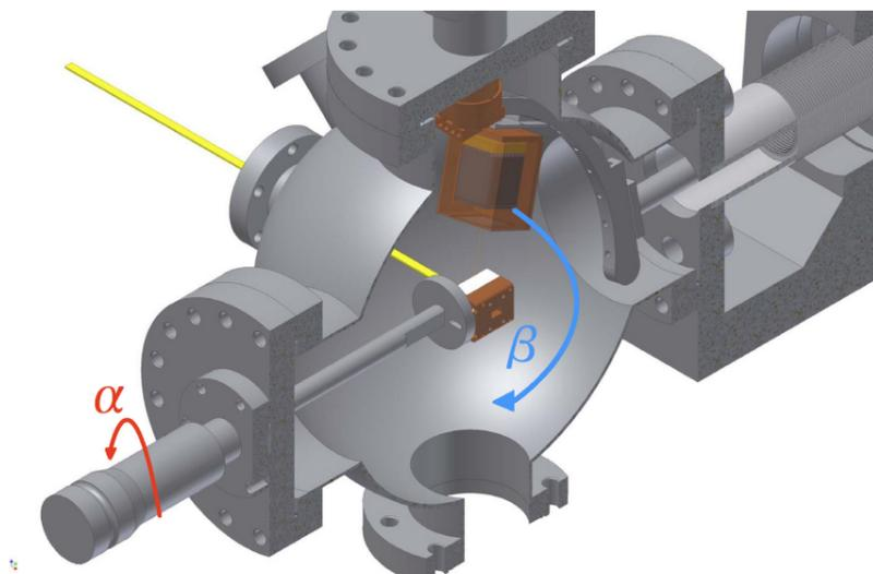
*Fig. 2 A cutaway view of the vacuum chamber, with unscaled angles labelled. (Aprile et al., 2009)*
