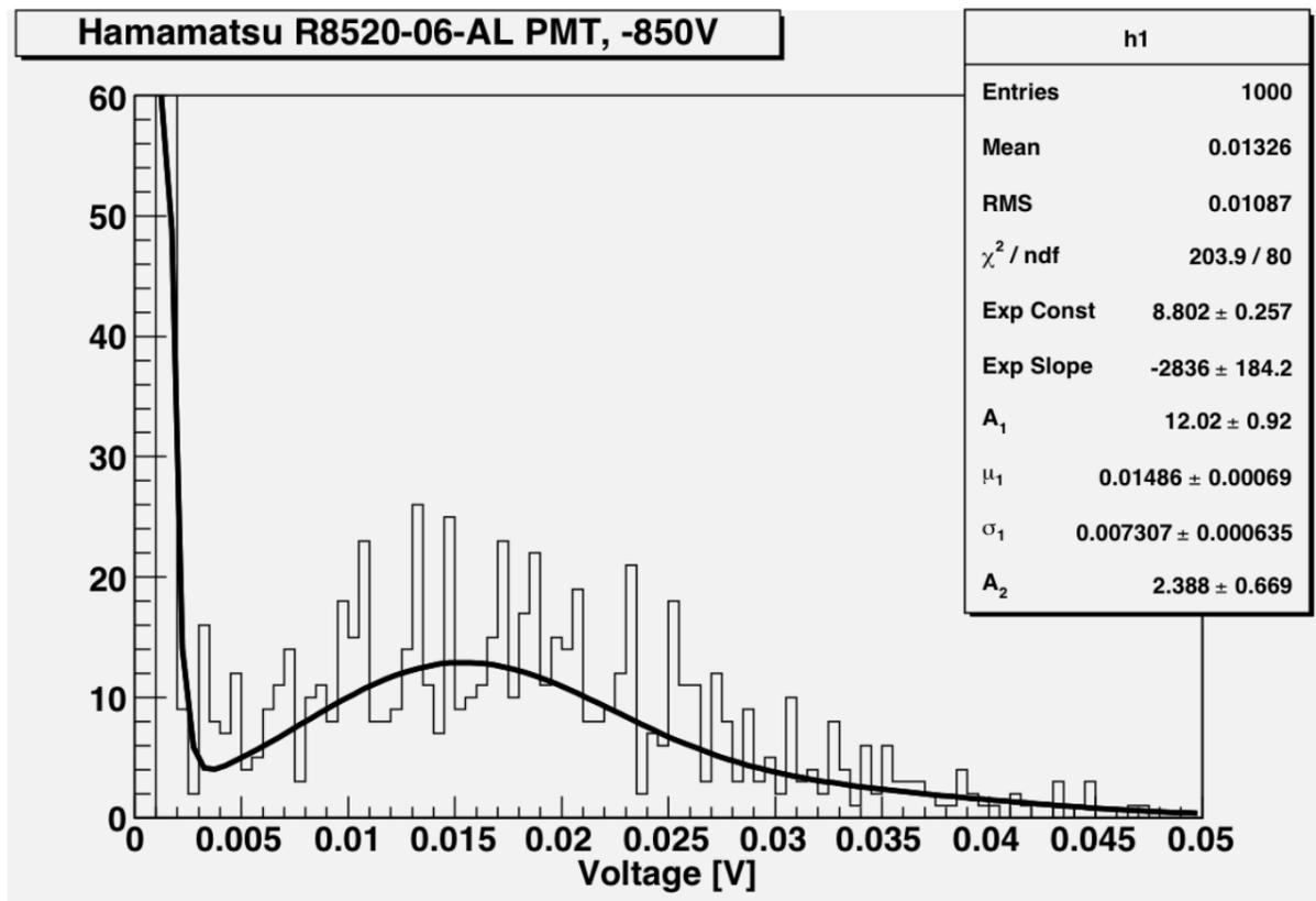
Fig. 4 SER spectrum for Hamamatsu R8520-06-AL PMT
