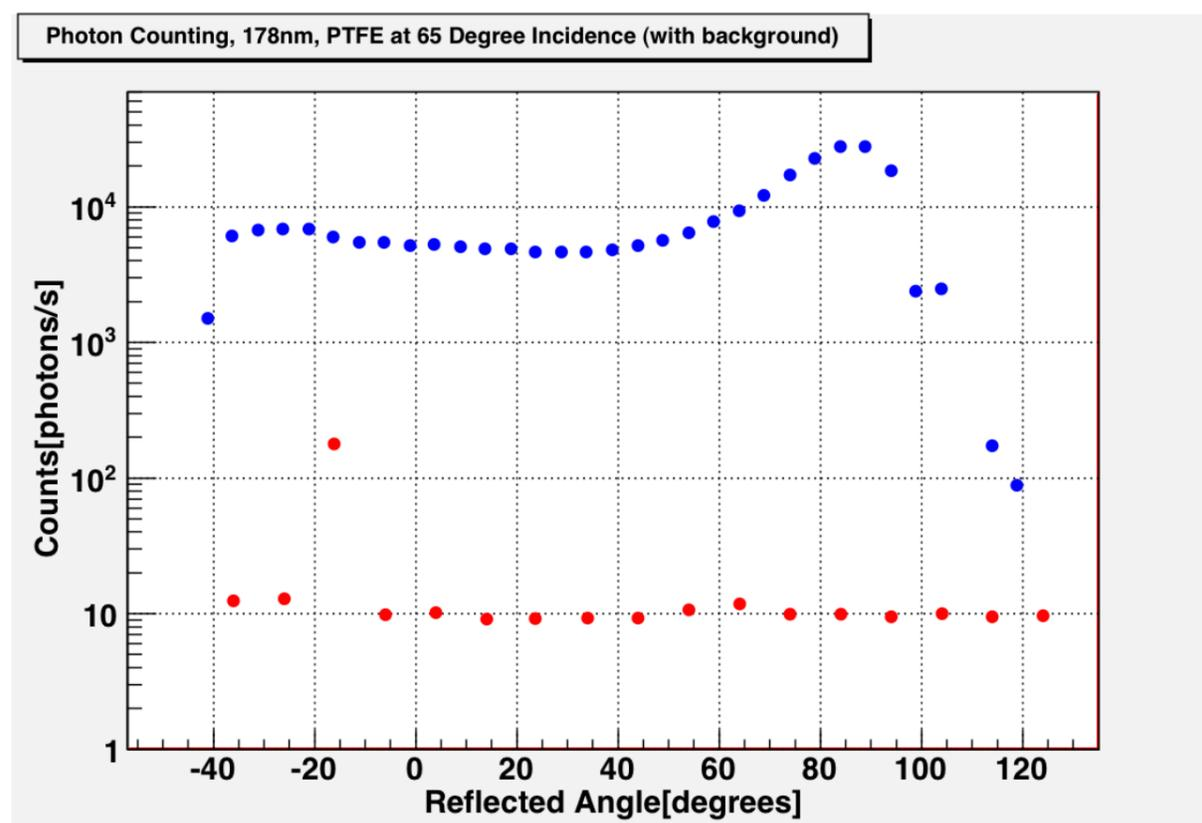
Fig. 3 Reflection measurement with photon counting method for  $65^\circ$  incidence,  $\lambda=178\text{nm}$ , with background
