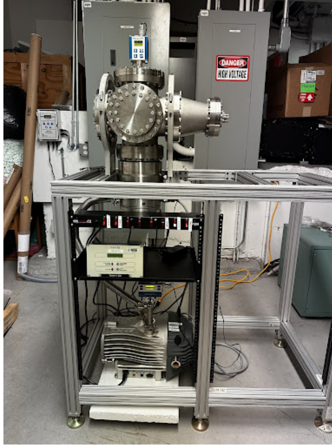
Figure 11: Metal stand after modifications and with a vacuum system mounted, including a channeltron.
