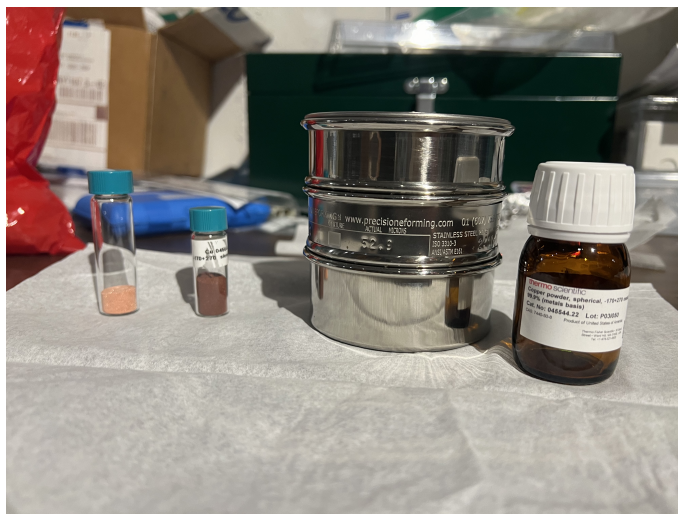
Figure 6: From left to right: Reduced and sieved Cu sample, Sieved CuO sample, sieve stack (90 micron screen on top, 53 micron screen in middle, catcher tray on the bottom), and the CuO sample as it was purchased.
