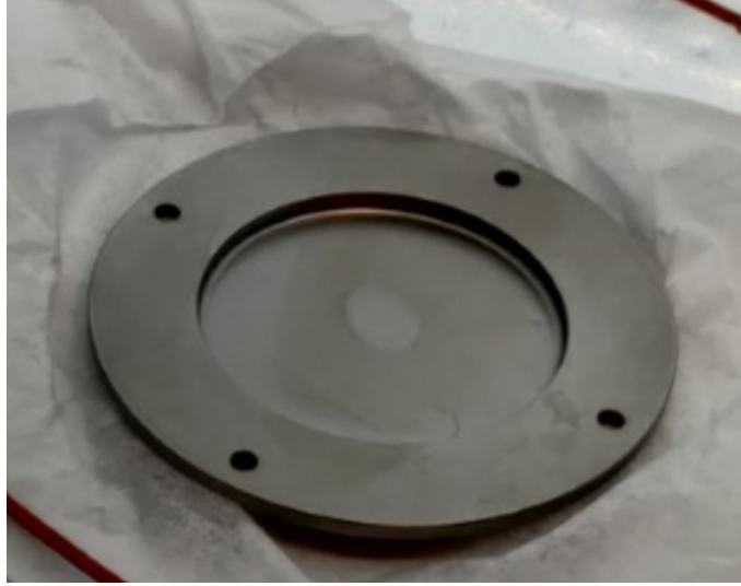
Figure 7: The sample cup after being irradiated by the ion beam, and hit with electrons from the flood gun. The smaller light mark in the center is due to the ion beam, and the larger darker mark is from the flood gun electrons.
