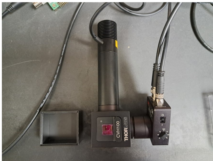
Figure 1: Fluorescence intensity measurement setup. An LED at the peak excitation wavelength is attached to a cuvette holder with the sample. Light shines through a filter and is received by the detector on the right.
