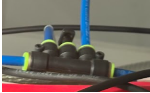
Figure 9: Main nitrogen connector suspected of leaking in the instrument control supply line.
