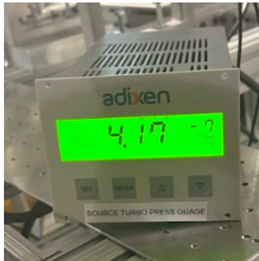
Figure 3: Turbo pump pressure gauge used to monitor vacuum levels near the ion source during staged leak isolation diagnostics
