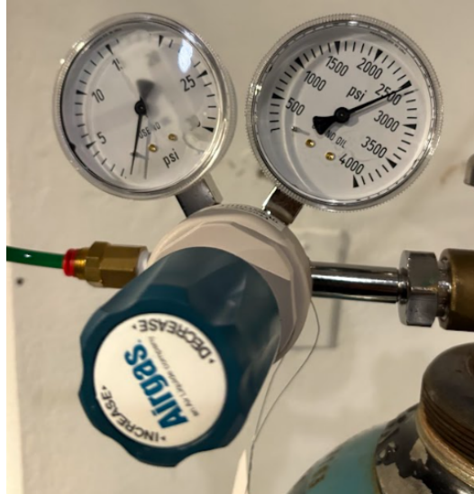
Figure 4: Nitrogen gas regulator gauge used to isolate and test supply pressure to the ion source.
