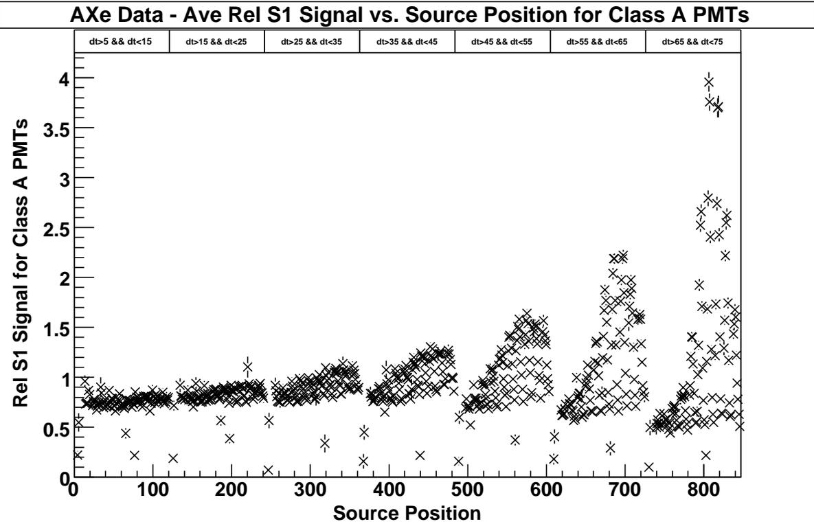
FIG. 9: The S1 signal from the AXe data, relative to the center of the detector and averaged for all class A PMTs, as a function of the source position.
