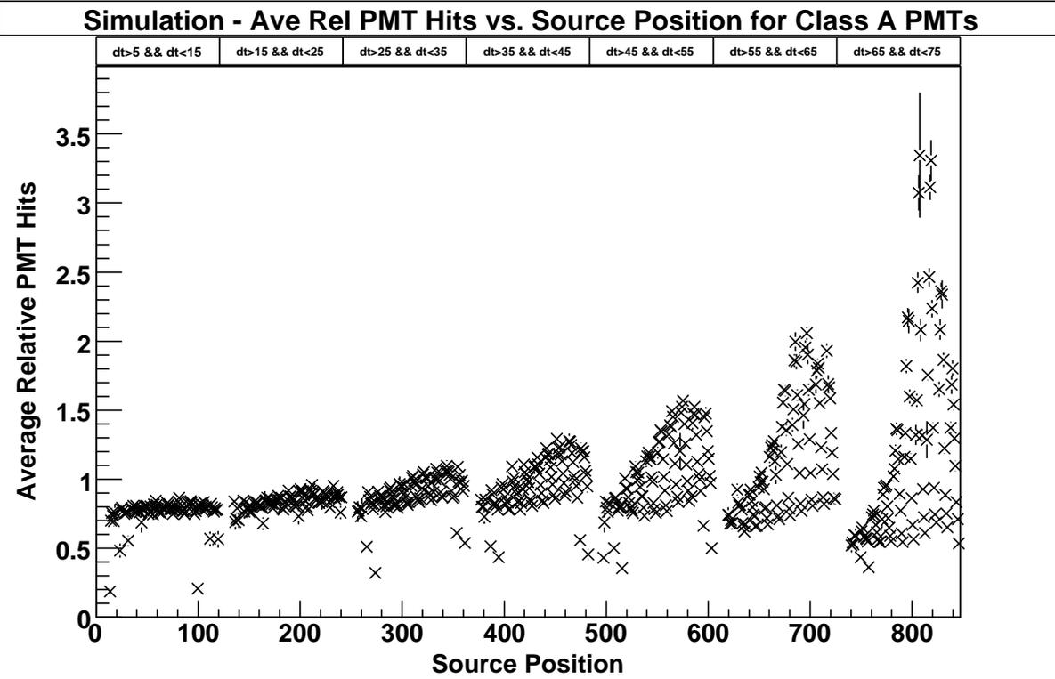
FIG. 10: The S1 signal from the simulation, relative to the center of the detector and averaged for all class A PMTs, as a function of the source position.
