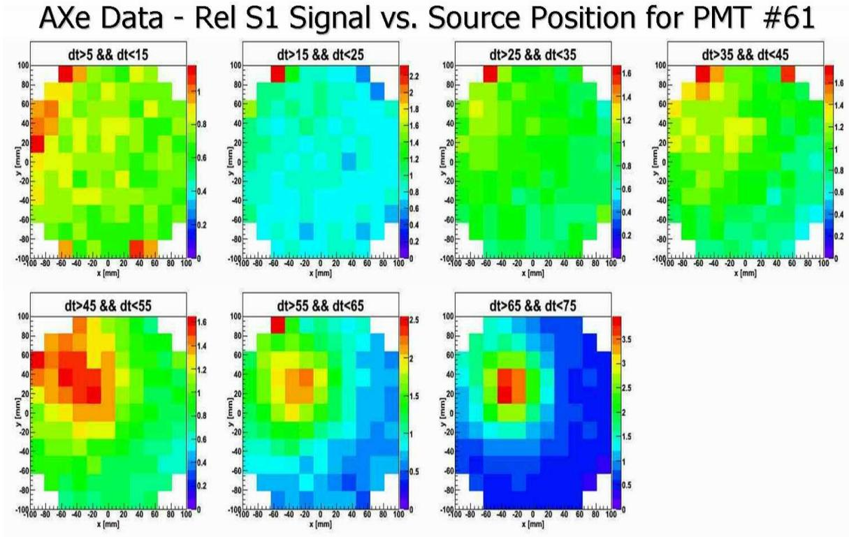
FIG. 6: The S1 signal from the AXe data, relative to the center of the detector, as a function of the source position for PMT #61. Each plot is of a different layer in the  $z$  direction.
