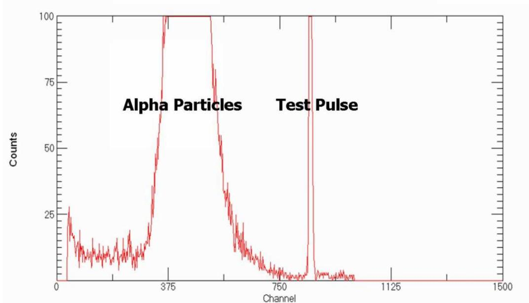
FIG. 13: A sample spectrum showing the direct  $\alpha$ -peak and test pulse for a bias of -260 V.
