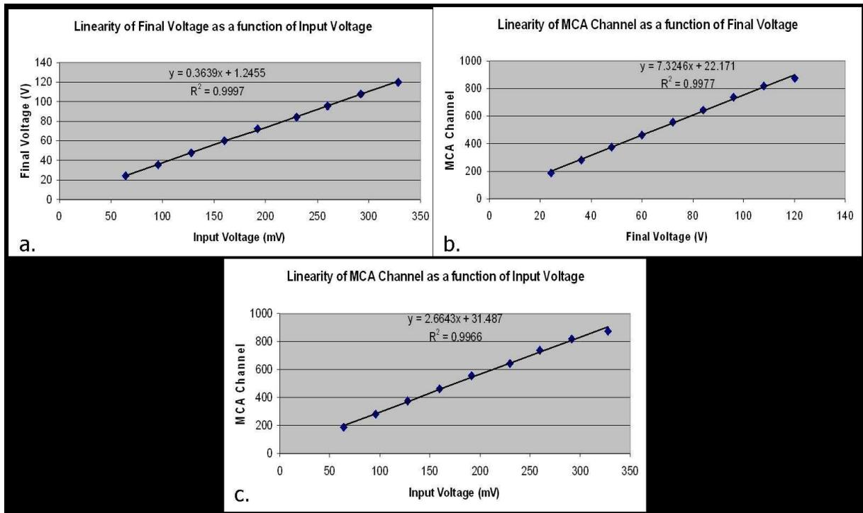
FIG. 12: a. The voltage out of the amplifier (final voltage) as a function of the voltage into the preamplifier (input voltage). b. The MCA channel as a function of the final voltage. c. The MCA channel as a function of the input voltage.
