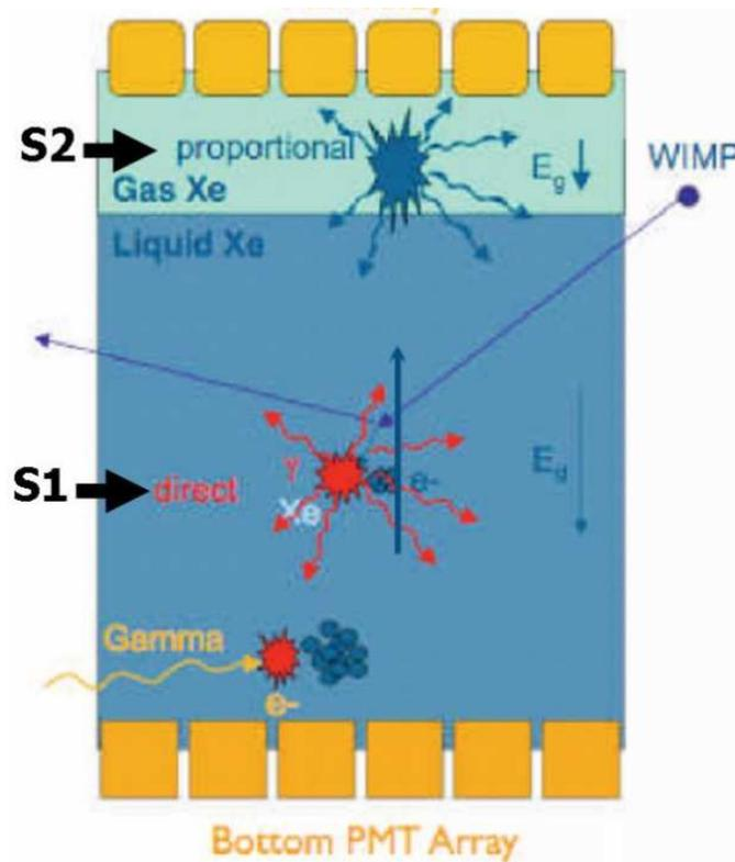
FIG. 3: Illustration of the possible signals from the liquid xenon time projection chamber.
