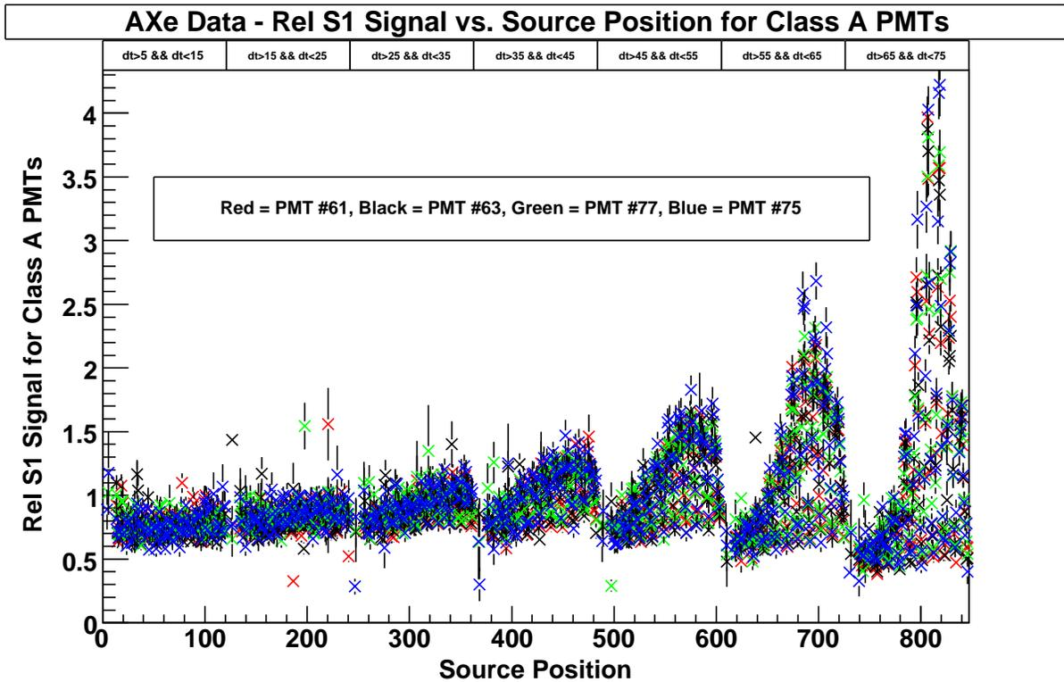
FIG. 8: Comparison of the S1 signal from the AXe data, relative to the center of the detector, as a function of the source position for class A PMTs.
