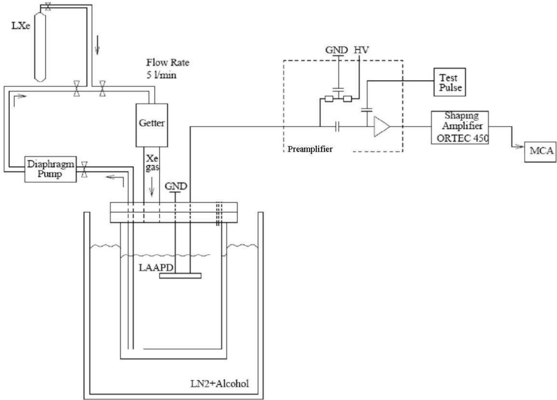
FIG. 11: Schematic drawing of the detector and electronics for the APD tests.
