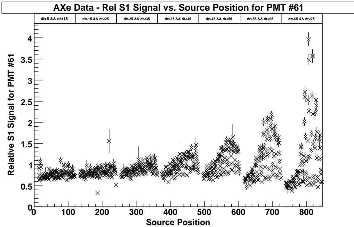
FIG. 7: The S1 signal from the AXe data, relative to the center of the detector, as a function of the source position for PMT #61.
