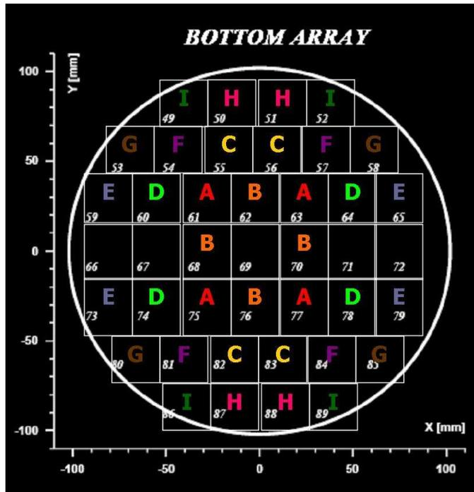
FIG. 5: Bottom array of PMTs and their classes.
