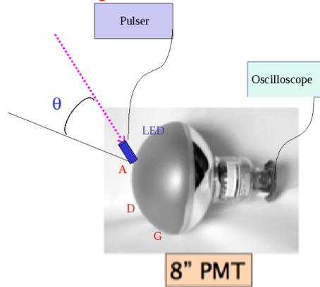
Figure 3: Incidence Angle Setup
