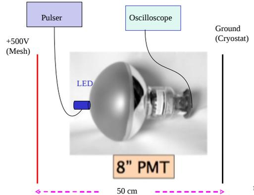
Figure 6: Electric Field Setup
