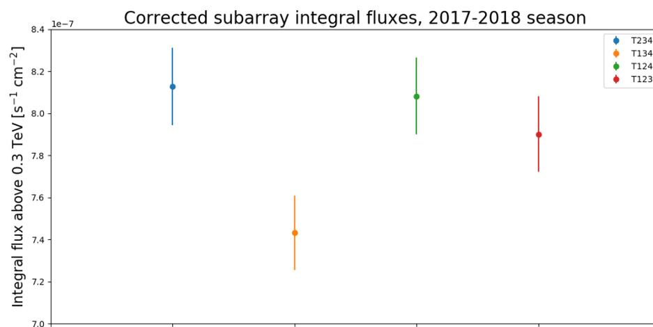
Figure 7: Corrected integral Crab fluxes for individual VERITAS subarrays.
