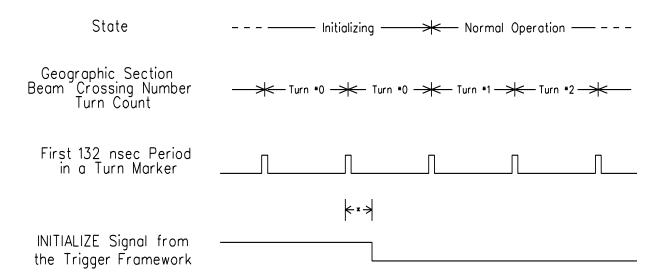
\* Note: The Trigger Framework guarantees that the delay between the "First 132 nsec Period in a Turn Marker" and the falling of the INITIALIZE Signal will be between 10 and 20 periods of 132 nsec (i.e. between 10 and 20 ticks).
