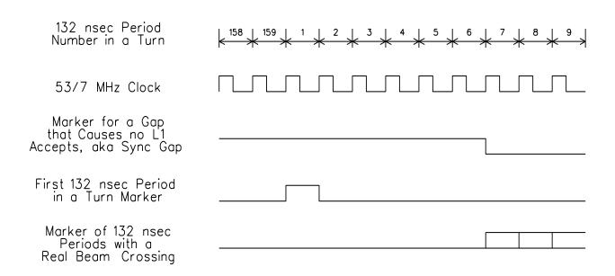
Figure 1: Serial Command Link, Clock Signals and Markers, Two Time Scales
