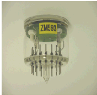
Fig. 13. The first attempt by Hamamatsu at permanently sealed gaseous detector with Bialkali photocathode and the Micromegas, filled with the P-10 gas.
