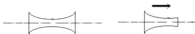
Figure 3 The symmetric (right) and the asymmetric spray nozzle (the arrow indicates the normal direction of the spray)
