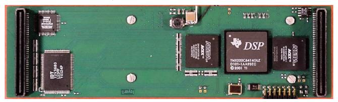
The 6414 PU in the ROD Demo format has been designed during November 2001 jointly by Nevis and LAPP.
